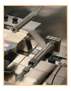
Unique, quick change cover tape guide makes it easy to change tape sizes without the need for additional tooling.
