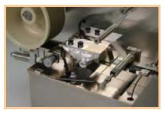
Advanced multi-mode sealing station with dual pressure and temperature controls.
