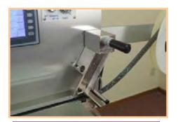
Optional de-tape module removes old cover tape from a finished reel and simultaneously applies a new cover tape without a reduction in throughput.
