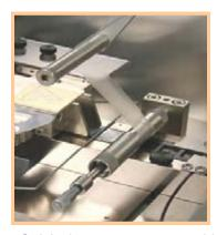
, Quick change cover tape guide makes tape size change easy. No tooling change needed.
